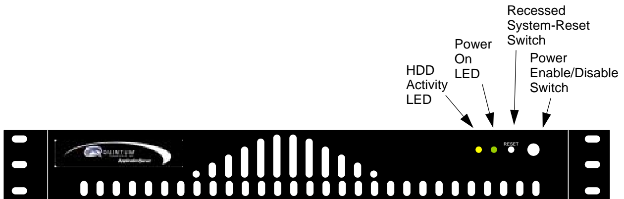
Figure 1 ApplicationServer - front panel
