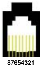
Figure 2 10/100 Ethernet LAN Port Pin Order
